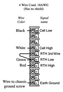
Figure 7-14 Terminal Designations for Conductivity with Integral Cable
